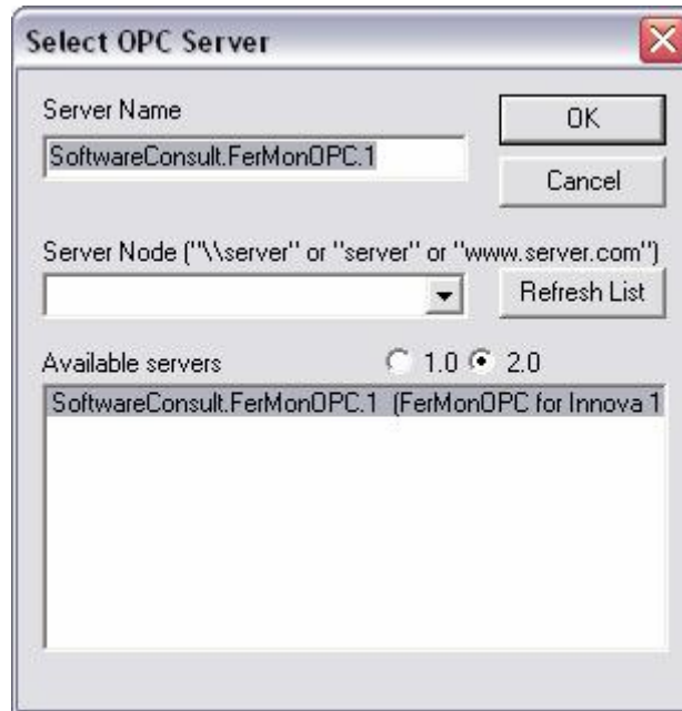
Figure 7: Connecting to FerMon using an OPC client can often be done by selecting the ID from a list or by typing it in a text field. Remember to specify which network host to connect to, if connecting over a local area network (LAN).
